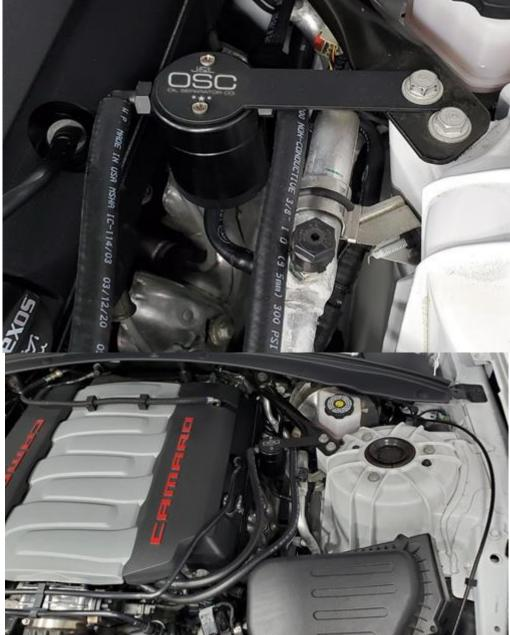
To properly clean the filter in the Oil Separator, spray any degreaser or solvent through it and let it air dry. Clean it every 10,000 miles.
